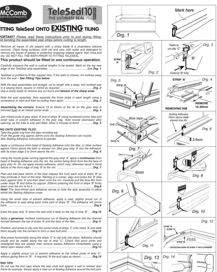
installed. Ensure Adhesive does not bond the strips or Caps together! Please Note! Durability is the key element in TeleSeals design & development. Without control over the products installation or use however, we cannot provide guarantees nor accept responsibility for the failure or damage resulting. This does not affect your statutory rights McComb Developments maintain the right to make modifications or improvements to its products with or without prior notification
